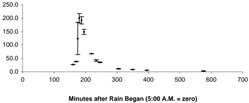
Figure 12. Measured turbidity of water samples taken from Terciopelo Stream during and after heavy rainfall on June 28. (mean  $\pm$  SE, n=3)
