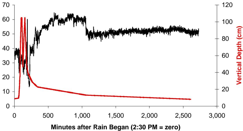
Figure 5. Velocity and vertical depth of Terciopelo Stream after heavy rainfall on July 24, 2007. Velocity (m/min) is shown in black and vertical depth (cm) is shown in red. Storm duration is recorded to be 150 minutes.
